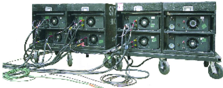
SB7K Ballasts in typical road configuration
