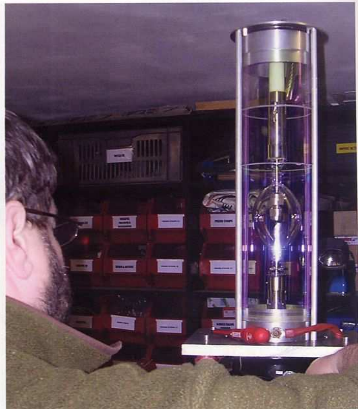
Yves Colombatto inspects a 7kW xenon internal "illuminator" that he designed to illuminate the heart of the sphere for a spectacular translucent effect.
