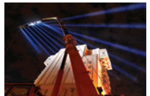
Backstage of the Tower of Terror: 12 rising xenon sources used from spot to flood.
