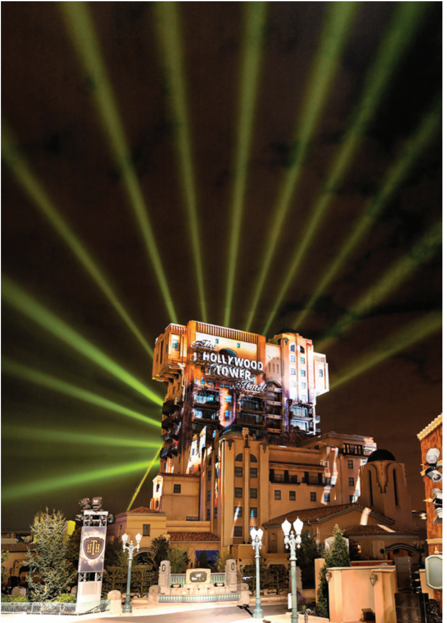
Disney Tower of Terror illuminated in spot and flood with a large pack of xenon Syncrolite SXB-5/2s a typical 'two in one' search/washlight system.
